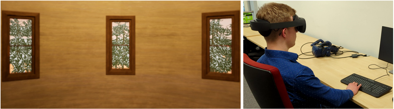
Figure 8: Setup for the VR pilot study. Participants view one central window surrounded by two peripheral windows in VR. The peripheral windows are placed at an eccentricity of \theta = 32.5^\circ to ensure full visibility in the headsets field of view. Behind each window is a group of trees which is set into motion. Each of these groups is separate to allow differing physical velocities in each window. Participants used a keyboard to indicate when they felt the velocities diverging.
