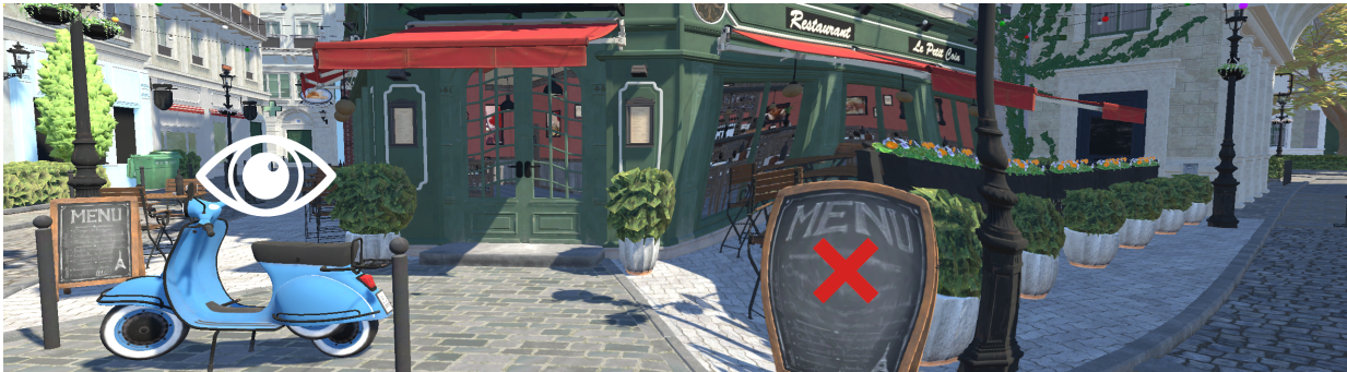
Fig. 1: A VR scene of a bistro, showing the warped space created by WarpVision in order to guide the visual attention to the menu board (highlighted by the red cross). The strength of the effect depends on eccentricity in the visual field determined by eye tracking (the current gaze position is represented by the eye symbol on the left).
