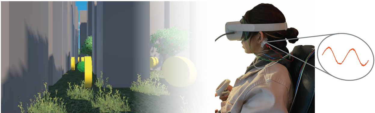
Figure 1: We present a novel scene-independent approach to mitigate motion sickness by desensitizing the vestibular system using semi-random Galvanic Vestibular Stimulation (GVS). Unlike existing scene-dependent methods that enhance vestibular feedback based on visual motion, our technique applies a low-frequency signal with mild stochastic modulation to disrupt natural vestibular responses. This avoids the discomfort commonly associated with fully stochastic (noisy) GVS while preserving its beneficial effects. The method operates independently of user motion or scene content, demonstrating potential for generalization beyond VR to real-world motion scenarios.
