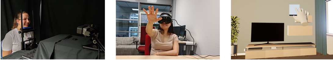
Figure B.1: We explore the use of electrical muscle stimulation to elicit eye blinks in VR users for instantaneous hand redirection. In a first eye-tracking experiment, we verify the reliability of triggering full eye closure with our novel stimulation model (left). In a second comprehensive VR experiment, we exploit muscle stimulation in conjunction with hand tracking to achieve imperceptible redirection (middle and right). Thereby, our method does not require eye tracking.
