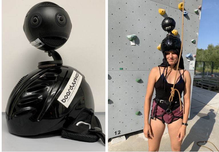
Figure E.4: Helmet carrying the 360° camera to capture the recordings for the experiment.
