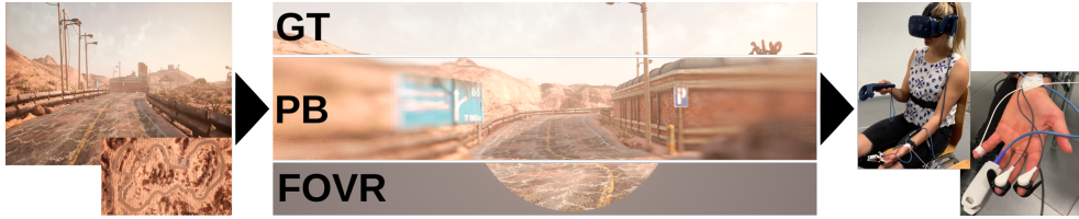
Figure D.1: This paper explores the impact of two different visual techniques – i.e., peripheral blurring (PB) and field of view reduction (FOVR) – to mitigate cybersickness in user-explorable game environments. Towards this goal, we conduct an experiment recording both self-reported (SSQ) and physiological (heart rate and electrodermal activity) data from our participants.
