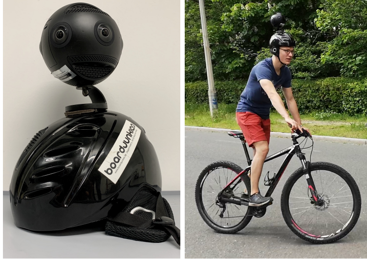
Figure A.4: Left: Helmet carrying the 360° camera to capture the recordings for the experiment. Right: Camera in action.
