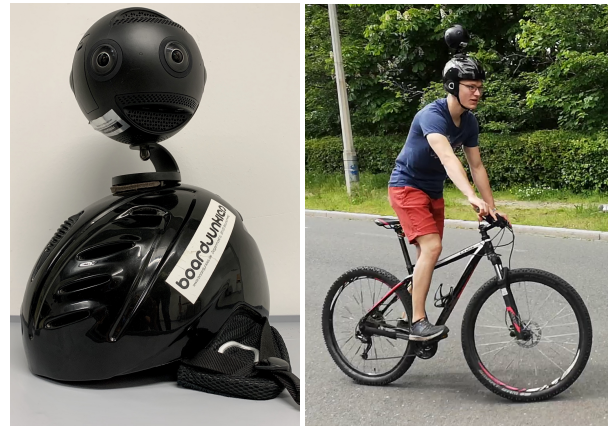
Fig. 4. Left: Helmet carrying the 360° camera to capture the recordings for the experiment. Right: Camera in action.
