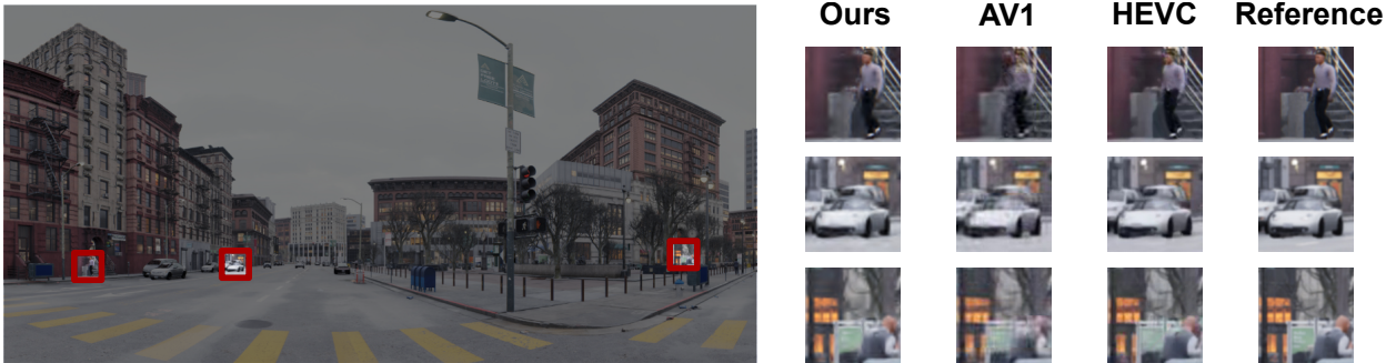
Fig. 1: In this paper, we propose a wavelet-based video codec that is able to load and decode the data of 360° videos viewport-dependently by exploiting the properties of the wavelet transform. While the quality is on par with state-of-the-art video codecs, we can achieve significantly faster playback times. Here, a visual comparison of our codec is given with HEVC, AV1 and the uncompressed reference. The samples are out of the computer-generated City video (left), all with 8k full-frame resolution.
